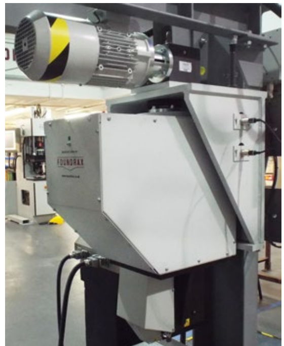
Type D Test Head module with actuation integrated into customer machine frame.
