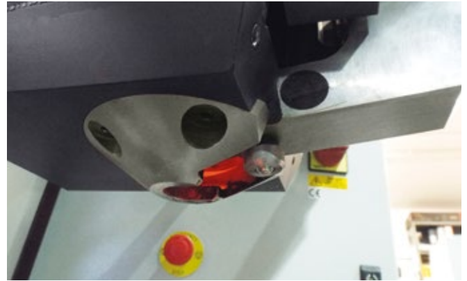
The illumination of the indentation requires no adjustment in use - whatever the material or hardness.
